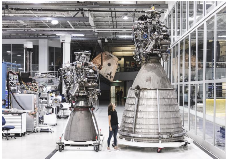
Figure 3. Raptor engine optimized for sea level operation (left) and vacuum operation (right) have the same throat diameter but vastly different nozzle diameters. Courtesy of SpaceX [23]
