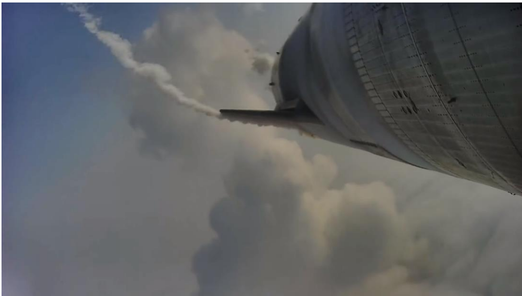
Figure 17. Image from SpaceX Starship SN15 High-Altitude Flight Test webcast showing flap deployment neutral position of about 45-degrees. Courtesy of SpaceX [16]
